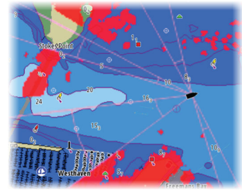
Radar overlay on a chart
